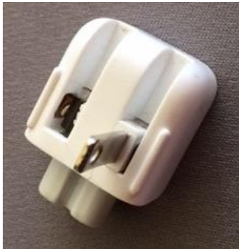
Power Adapter With Broken Blade
