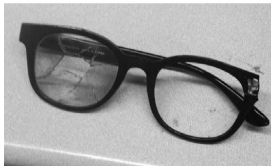
Photo 1 - Researcher's glasses after explosion. One lens and a temple bar have been blown away. The other lens is shattered.
