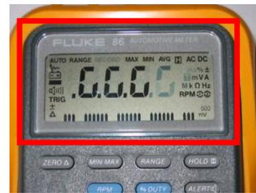
**6** Turn the meter on and confirm proper operation of the display.
