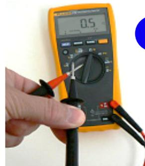
**7** Set meter to  $\Omega$ . Cross meter leads. Good leads will read in 0.1-0.5 ohm range. Bad leads will read OL. Jiggle the leads and watch the reading for loose connections or internal wire damage.
