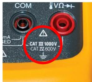
**3** Both the meter and the leads should be NRTL-listed, double-insulated and CAT-rated.
