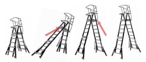
BEGIN FROM THE SMALL A-FRAME POSITION. STAND TO ONE SIDE OF THE CAGE; UNLOCK BOTH ROCK LOCKS ON ONE OUTER SECTION, (WHEN EXTENDING THE CAGE YOUR HANDS MUST ALWAYS BE ON THE OUTSIDE OF THE OUTER SECTION), PLACE ONE HAND ON THE PLATFORM OR UPPER INNER RAILS AND PUSH THE INNER SECTION AWAY FROM YOU TO EXTEND THE CAGE. ONCE YOU HAVE REACHED THE DESIRED HEIGHT, LINE UP THE INNER AND OUTER RUNGS, THEN LOCK BOTH ROCK LOCKS.
